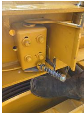
P81.11: Luff up limit switch on luffing drum disconnected
