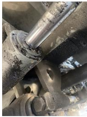
P22.2: Leak on cylinder 5th axle back passenger side
